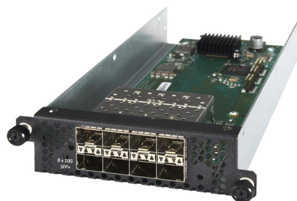
(I/O Module with 8 x 1/10 SFP+)
