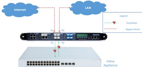
**Figure 2: Bypass Mode**
